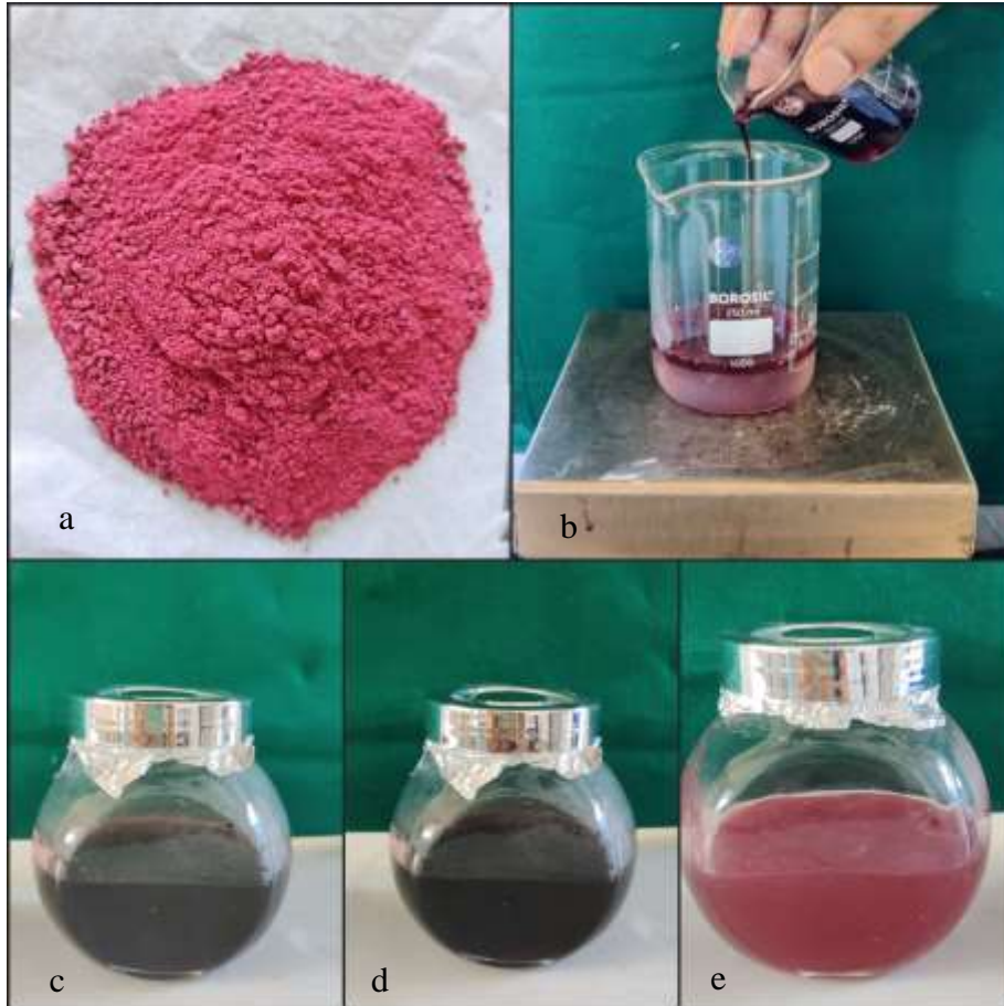
Figure.1: a) cranberry powder; b) preparation of cranberry hydrogel; c,d and e) final product of cranberry hydrogel in 1%, 2.5% and 5% respectively.
