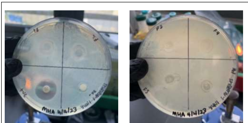
Figure 3: First zone of inhibition for positive control, negative control and all 6 film formulations
