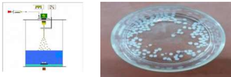
Figure1: The preparation of composite (clay/chitosane bead).
