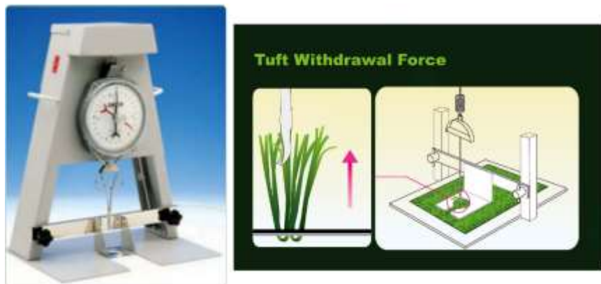
Figure 1. Pile withdrawal test device
