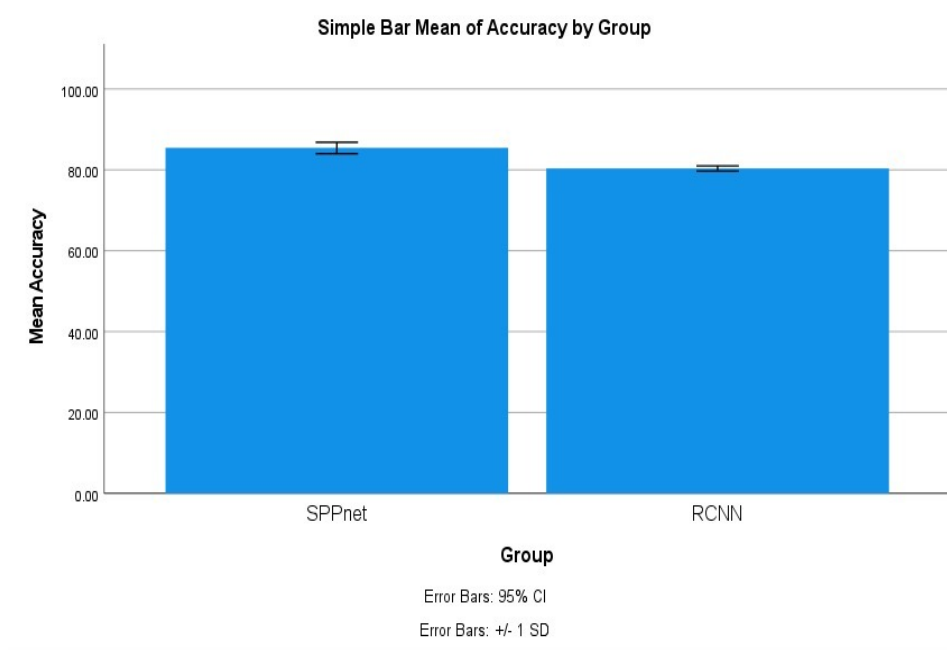
Fig. 1. Comparison of regional proposal network based SPPnet in terms of mean accuracy. As the graph shows, the mean accuracy of the SPPnet is greater than the R-CNN. Graphical representation of the bar graph is plotted using group id as X-axis SPPnet vs R-CNN, Y-axis displaying the error bars with mean accuracy of detection +/- 1 SD.
