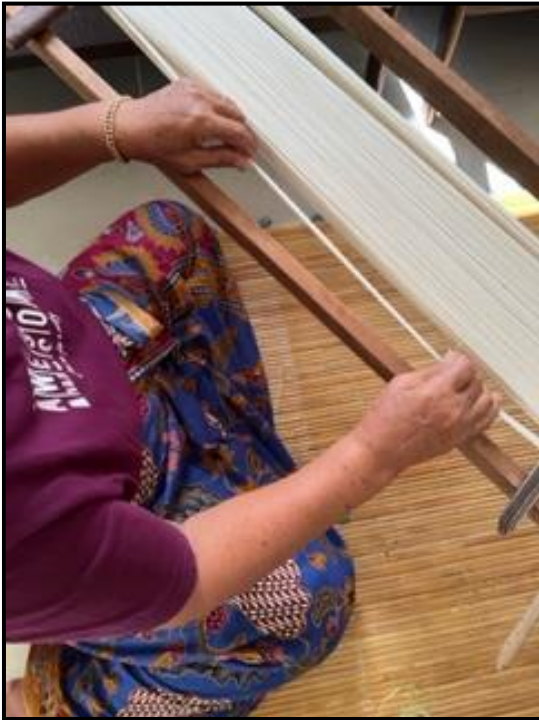
Fig. 13: Ngirit technique where a thread is horizontally pulled, stretched, and knotted before the dye is applied.
