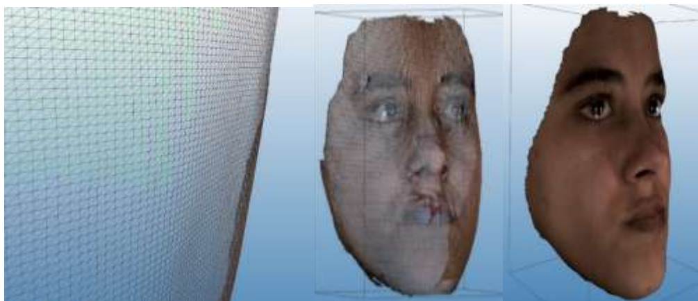
Figure 1 left image represents a magnified part of the polygonal mesh, middle image is the outline of the full polygonal mesh, right image represents skin textured mapping of the face over the polygonal mesh
