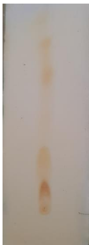
Figure 3: TLC of methanolic extract in chloroform: methanol (5 : 5)
