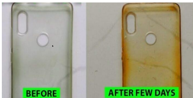
Fig.2. Color changing because of high-temperature
