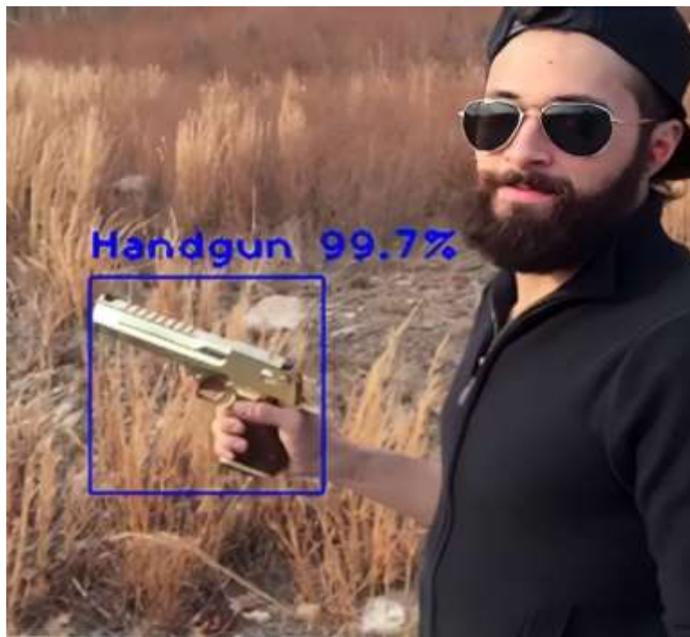
Fig.10(An Example of accurate weapons detected in a frame)
