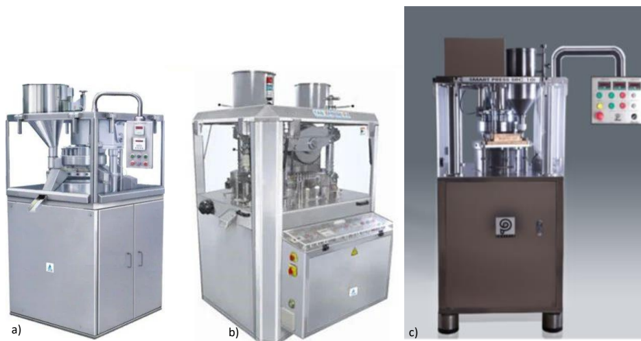
Figure 4. Different Types of Tablet Compression Machines a) Single-sided tablet press b) Double-sided tablet press c) Bilayer tablet press with displacement monitoring
