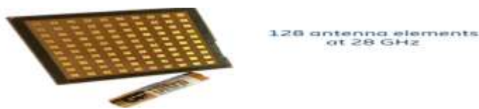
Figure 12: MIMO antenna with 128 antenna elements at 28GH
