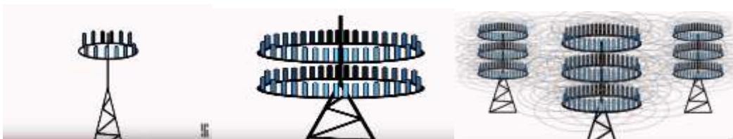
(a) MIMO Antenna (b) Massive MIMO (c) Massive MIMO with small cells
