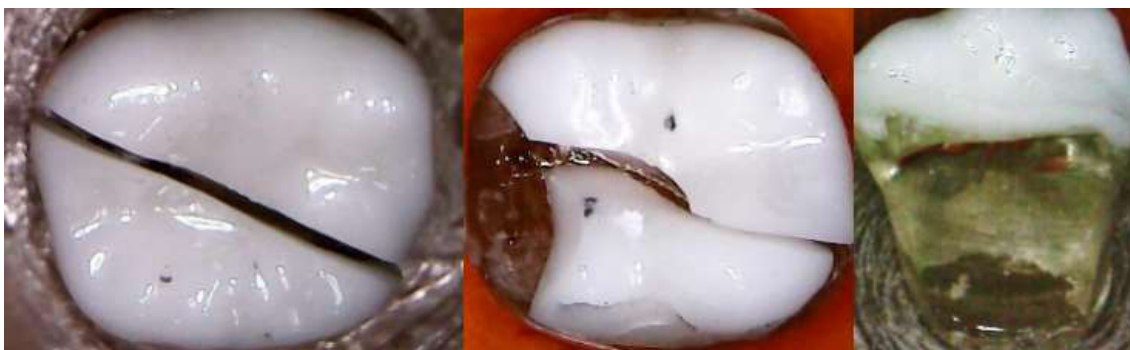
Figure (7): Descriptive digital microscopic images showing the three detected different failure patterns :(A) Mode I, (B) Mode II and (C) Mode III.
