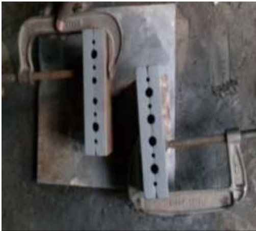
Fig.1. Cast iron mould with C-clamp attachment
