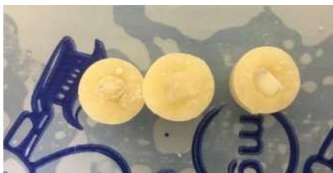
Figure (2) dentin specimens embedded in acrylic resin molds.
