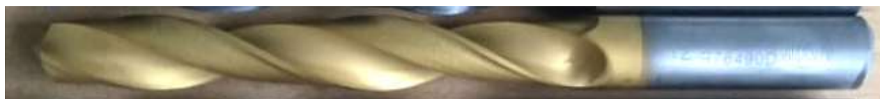
Fig. 2. High-speed steel (HSS) twist drill bit (10 mm) with high heat resistance and easily machinable, widely used for application for drilling. HSS is the most commonly used cutting tool in industries.
