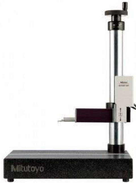
Fig. 5. Surface testing machine of Mitutoyo SJ-410 has 0.001Micron least count
