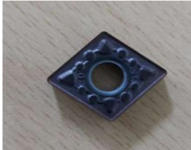
Fig. 3. High Speed Steel Tool, Tool include the thickness 4.8mm, Corner radius 0.4mm, Fixing hole diameter - 3.81mm
