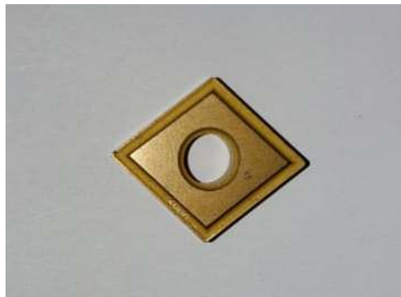
Fig. 2. Aluminium Chromium Nitride (AlCrN) coated Tungsten carbide Tool. Tool include the thickness 4.8mm, Corner radius 0.4mm, Fixing hole diameter - 3.81mm
