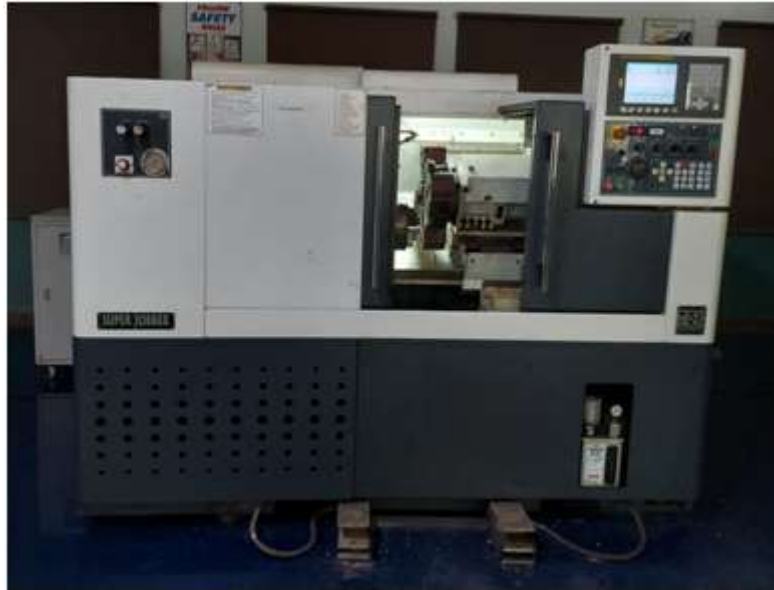
Fig. 1. CNC turning Machine center - Specifications: Swing carriage - 260mm, Maximum turning diameter - 290mm, Maximum turning length - 400/500mm, Swing bed - 500mm, Max spindle speed - 4000 rpm, no of stations - 8, Chuck size - 200/250mm
