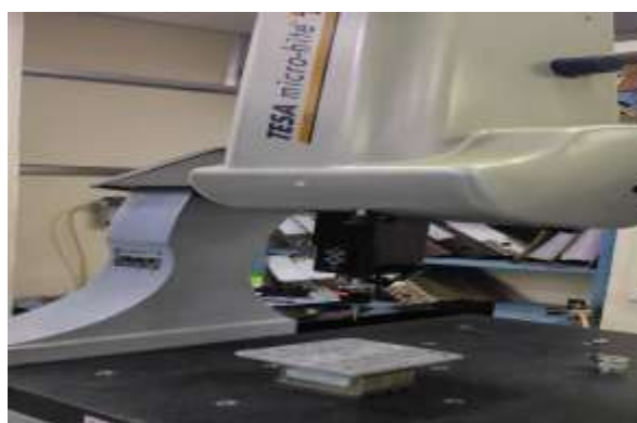
Fig. 2. During the Measurement of Cylindricity Tolerance Cylindricity Tolerance
