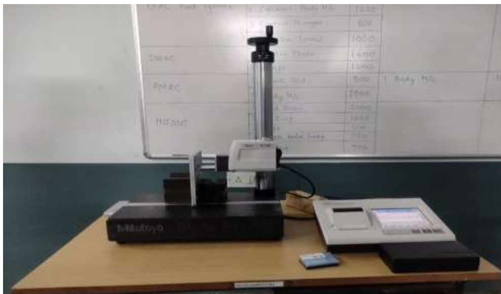
Fig. 1. During the Surface Roughness Testing
