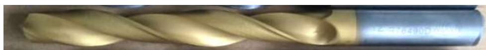
Fig. 2. Novel Titanium Carbonitride coated on HSS twist drill bit (10 mm) having yellow refractory coating on High-speed steel that improves hardness, wear resistance and gives more tool life.
