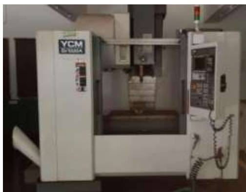
Fig. 3. YCM EV1020A CNC machining center. Specifications: Maximum spindle speed- 4000 rpm, Cutting speed- 150 m/min, Feed rate- 0.50 mm/min, drill depth- 30 mm, Swing over bed- 500 mm, Swing over carriage- 260 mm, No. of Stations- 8, Distance between centers- 425 mm.
