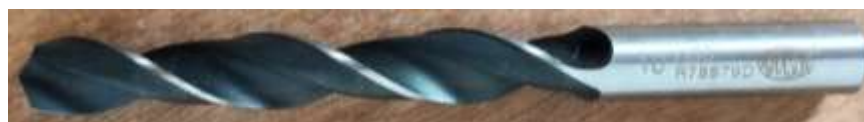
Fig. 1. High-speed steel (HSS) twist drill bit (10 mm) with high heat resistance and easily machinable, widely used for application for drilling. HSS is the most commonly used cutting tool in industries.
