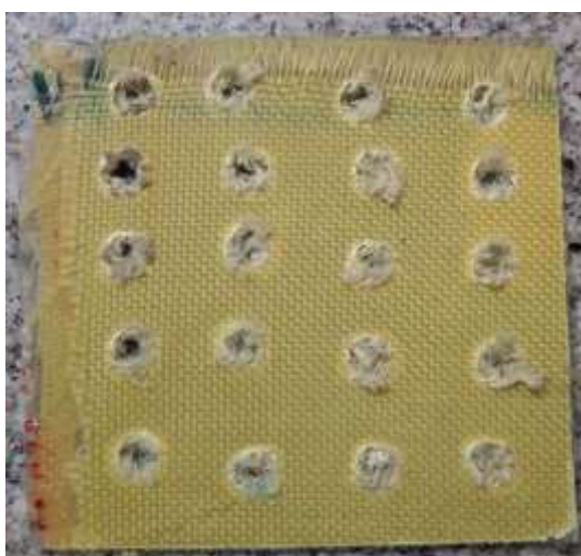
Fig. 2. Glass Fiber Reinforced With Aluminium Wire mesh after drilling
