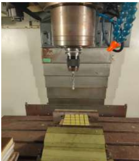
Fig. 3. CNC Drilling machine setup used for drilling of Glass fiber composite material
